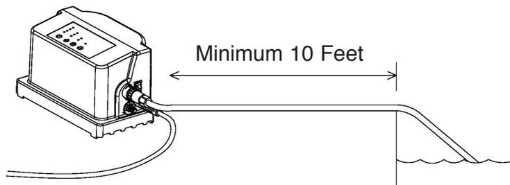
3. Connect the floating cable to the power supply control box. Use only the original Power Supply manufactured by Blue Torrent. Connect the floating cable to the control box as follow photo. Make sure they are connected correctly. (The fitting on the cleaner floating cable should be connected with the control box by turn at the clockwise direction).
