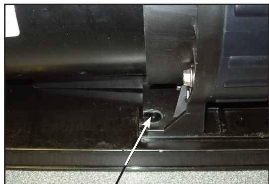
4B — Plastic pump housing mount
