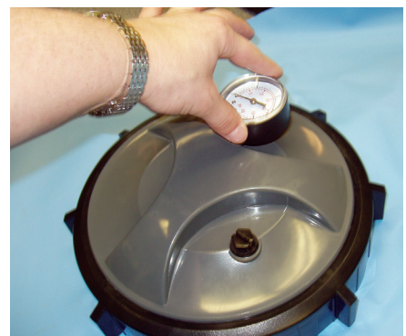
Figure 25b — Installing pressure gauge
