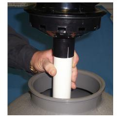
You CANNOT pull standpipe up to secure the valve. Pulling up can damage the laterals and cause sand to get sent back with water flow to pool.
