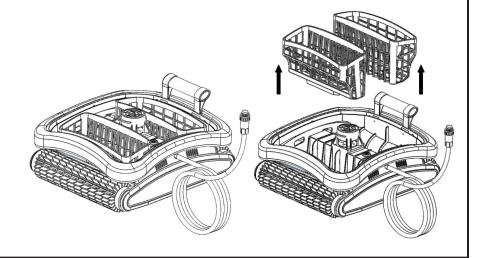
Flip the bucket assembly over to remove the debris & then rinse with a garden hose to remove small particles.
