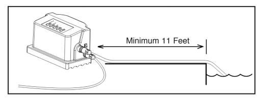
1. The The control box must be fixed at a minimum distance of 11 ft. from the edge of the swimming pool and minimum 8 ft. overtop of top edge of pool (outside Zone 1 defined in IEC 60364-7-702). Never operate the unit without fixing the control box first. The length of the standard CLEANER cable is 60 feet.
