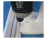
Screw Lower Base of Entrapment Barrier into bottom step of the Inside Portion of the Ladder with (2) #10 x 1-1/4" screws.
