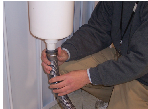
Figure 13 - Attaching hose to skimmer
