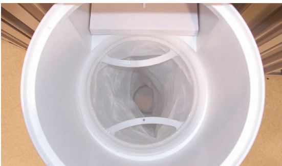
Figure 10 - Pre-Filter Bag installed in skimmer body
