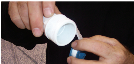
Figure 10 - Teflon tape hose adaptor
