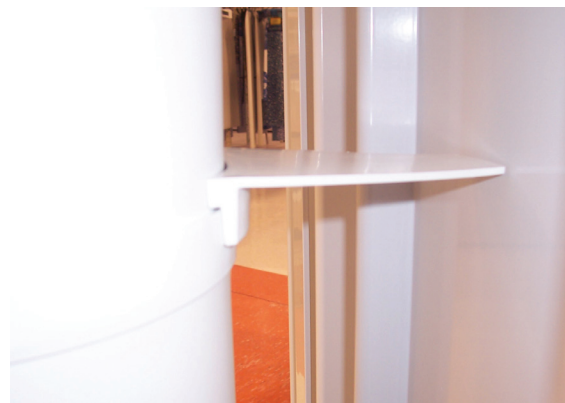
Figure 15 - Standoff installed, lip of standoff sits on lip of skimmer
