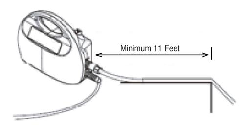
The control box must be fixed at a minimum distance of 11 ft. from the edge of the swimming pool and minimum 8 ft. overtop of top edge of pool (outside Zone 1 defined in IEC 60364-7-702). Never operate the unit without fixing the control box first. The length of the standard CLEANER cable is 60 feet.
