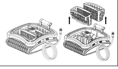
Reinstall the filter buckets in the right position, and make sure the concave of the filter bucket gets close to the inner edge of the robot, as shown.
