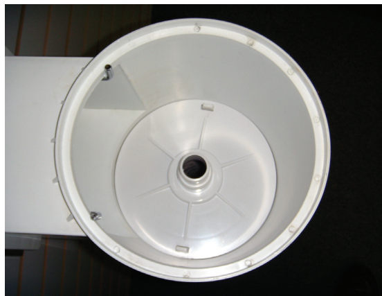
Vacuum Plate going onto Filter Cartridge
