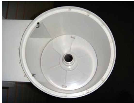
Vacuum Plate going onto Filter Cartridge
