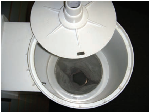
Vacuum Plate going onto Filter Cartridge
