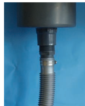
Figure 23b — Hose attached to thru wall skimmer
