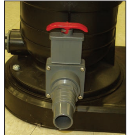
Figure 1 – Slide valve attached "TO POOL" on tank
