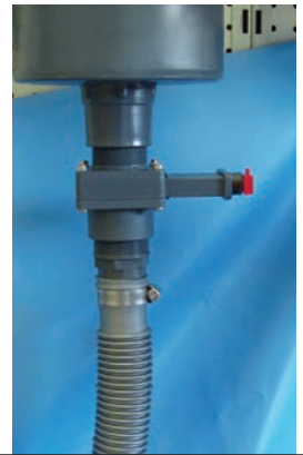
Figure 24 — Slide valve in closed position
