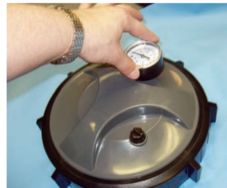
Figure 25b — Installing pressure gauge
