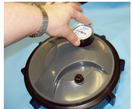
Figure 25b — Installing pressure gauge
