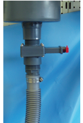
Figure 24 — Slide valve in closed position
