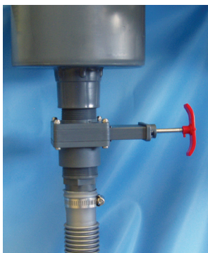
Figure 23a — Hose attached to thru wall skimmer with valve
