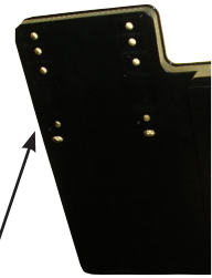
Figure 8a — Holes outside raised area
