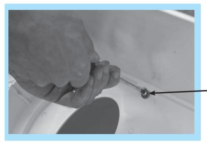
• Make sure you fasten step 4 to step 3 in all 4 points using the stainless steel washers with each screw.
